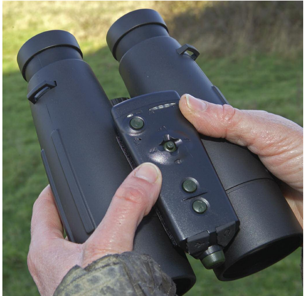
The RememBird solves the problem of the bulkiness and awkwardness of most other sound recording devices. It affixes conveniently between the barrels of your binocular, and it is easy to use in the field. Image courtesy of © Software Hothouse, Ltd.
