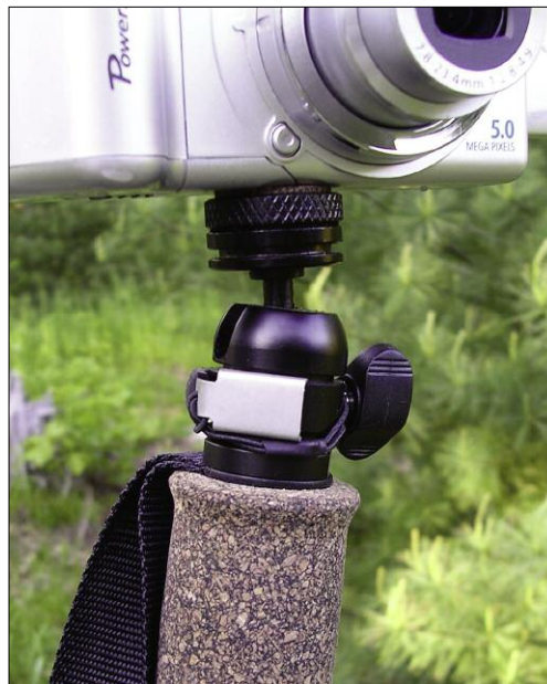
A unique feature of this combination staff-monopod-tripod is the fully-functional rotating ball head, allowing the user to alter the camera’s angle, such as on uneven ground. © Derek Lovitch.
